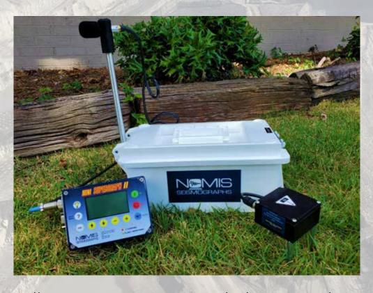
Our equipment allows you to monitor ground vibrations and air over-pressure with ease and accuracy. They can be used for most vibration and sound monitoring activities. This includes blasting operations, pile driving operations, construction equipment activity, environmental activity, ambient levels, and any other operation where a permanent record is needed. Our complete line of seismographs meets or exceeds ISEE standards
